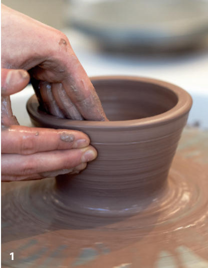
1 Center a ball of clay and open the form. Shape the bowl with a series of pulls.
