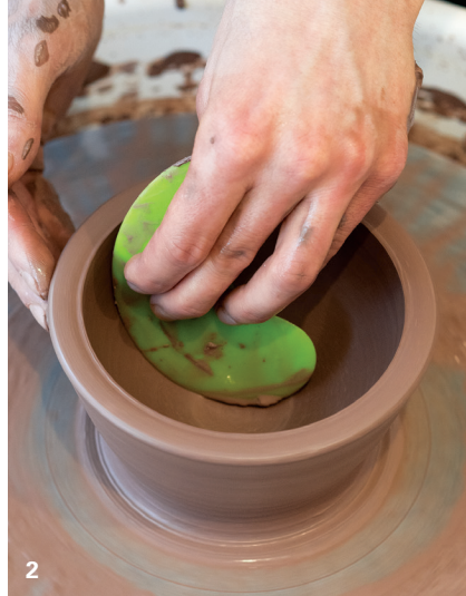
2 Remove excess slip from the interior (curved rib) and exterior walls (metal rib).
