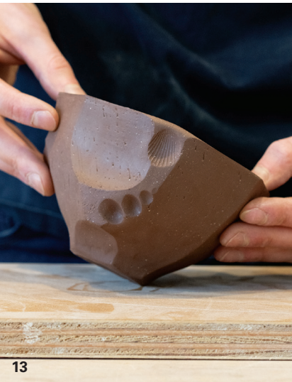
13 Roll the bowl at an angle to add a slight bevel to the foot to give it lift.
