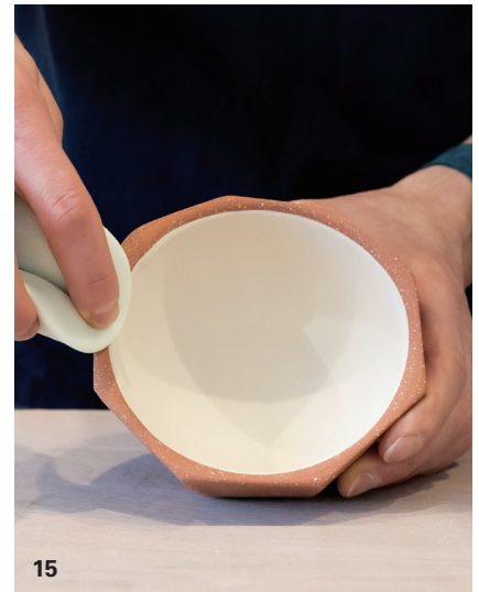
15 Use a damp sponge to wipe off any drips from the rim and the outside of the bowl.
