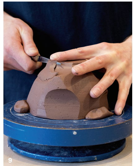
9 With a thin fettling knife, refine the shape and size of the foot.
