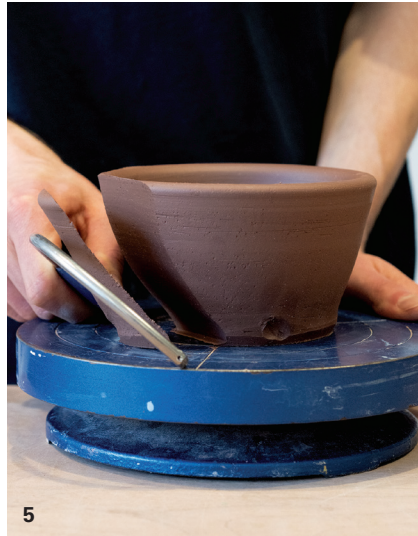
5 Move the bow outward and remove the piece of clay. Check for thickness.
