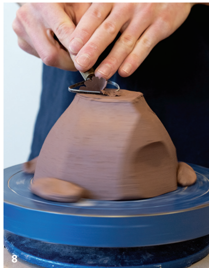
8 Trim the bowl on a spinning banding wheel so the foot is slightly concave.
